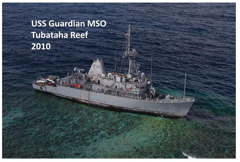
The coastal scale electronic chart supplied to USS *Guardian* was flawed due to human error on the part of the NGA. This error mis-located the Tubbataha Reef by 7.8 nautical miles from its actual location. NGA was aware of this error in 2011 and updated a smaller scale electronic chart, but failed to publish a correction for the larger scale chart that the USS *Guardian* was using when she ran aground.
