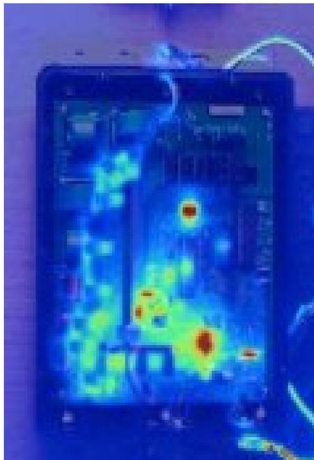
This time the main hotspots are the relay coils which are energised with DC (to the left) and RF sensing circuit and relay driver circuits (to the right).
