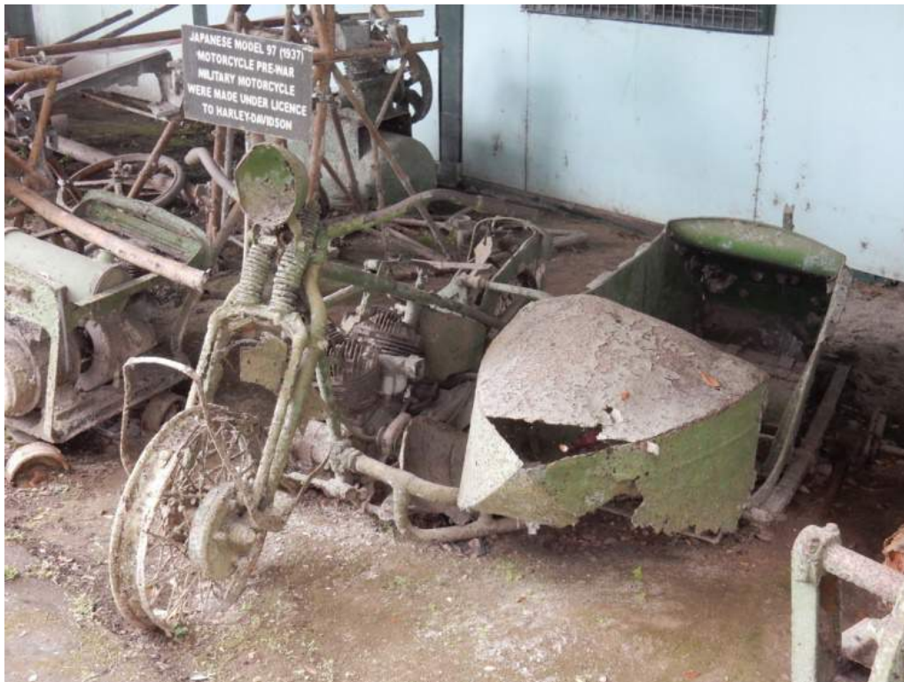
Japanese Model 97 Prewar military motorcycle with side car, licensed by Harley Davidson
