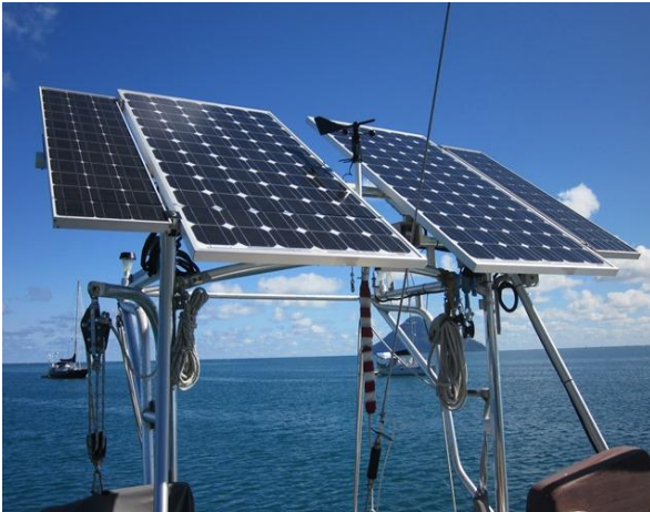
Fore and aft rotating solar array on the aft utility arch onboard a CSY 44.
