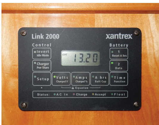
Our older Xantrex Link 2000 lead acid battery monitor which displays only total battery parameters
