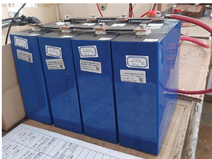
Four of our eight 3.2-volts per cell prismatic cells connected in parallel during top balancing. Grade A testing stickers are intact and show, among other things, capacity, voltage, serial number and date of manufacture
