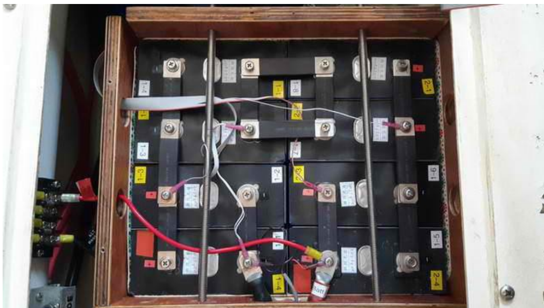
Our 8 LiFePO4 cells in their compression box in a 2P4S configuration.
