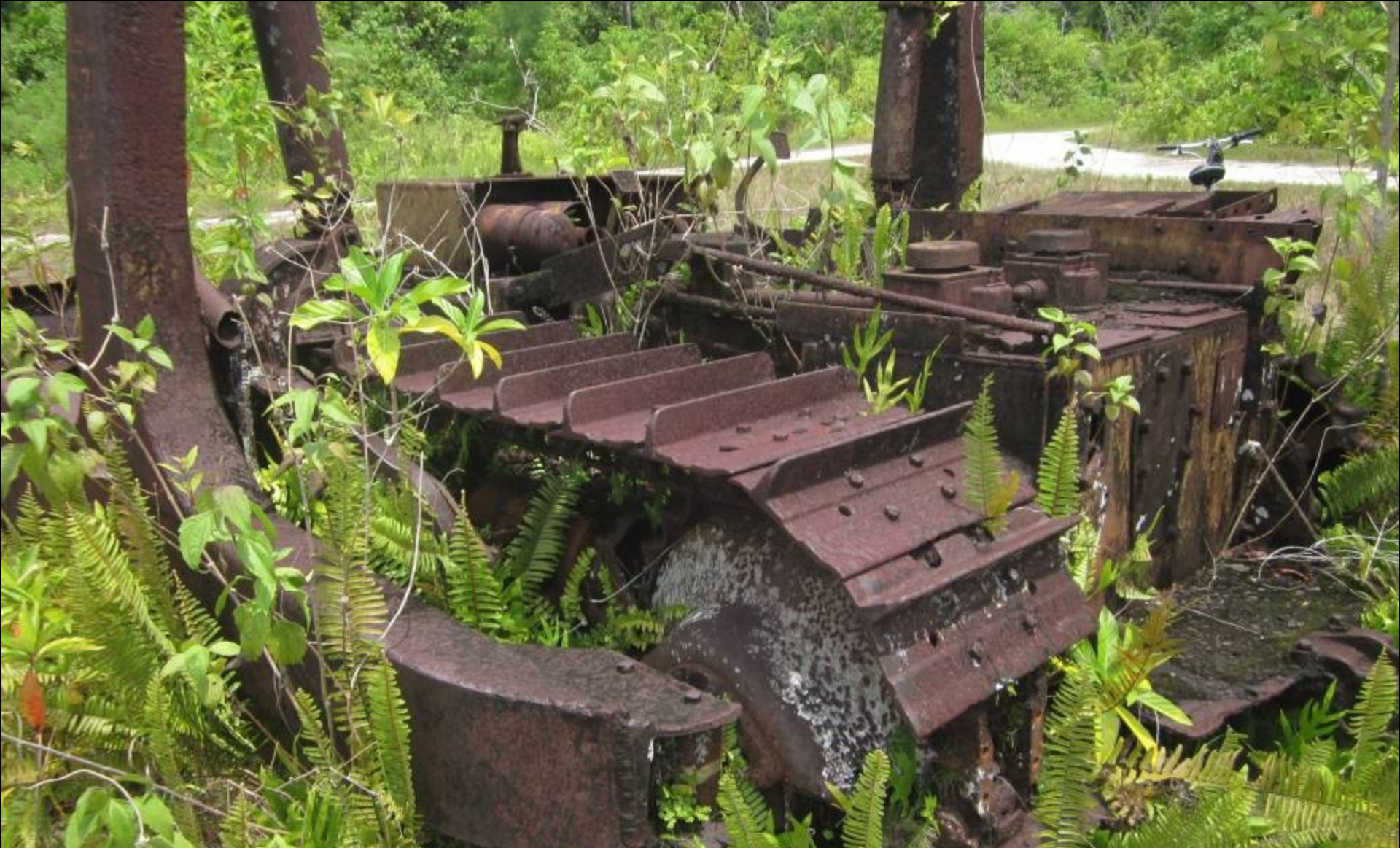
US Seabee construction International Harvester G-101 bulldozer, missing engine, marked 'CBMU 49'
