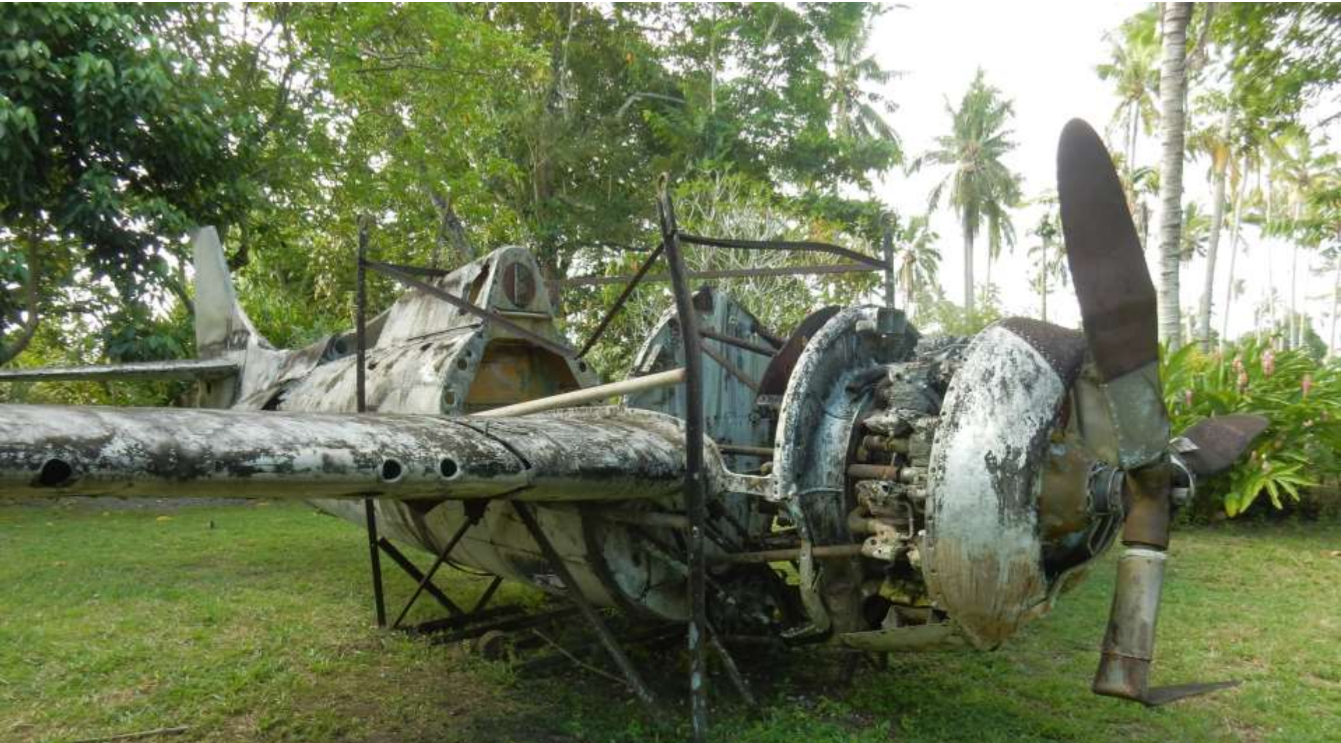
US F4F Wildcat with folding wing, note two holes in wing for 50 cal guns
