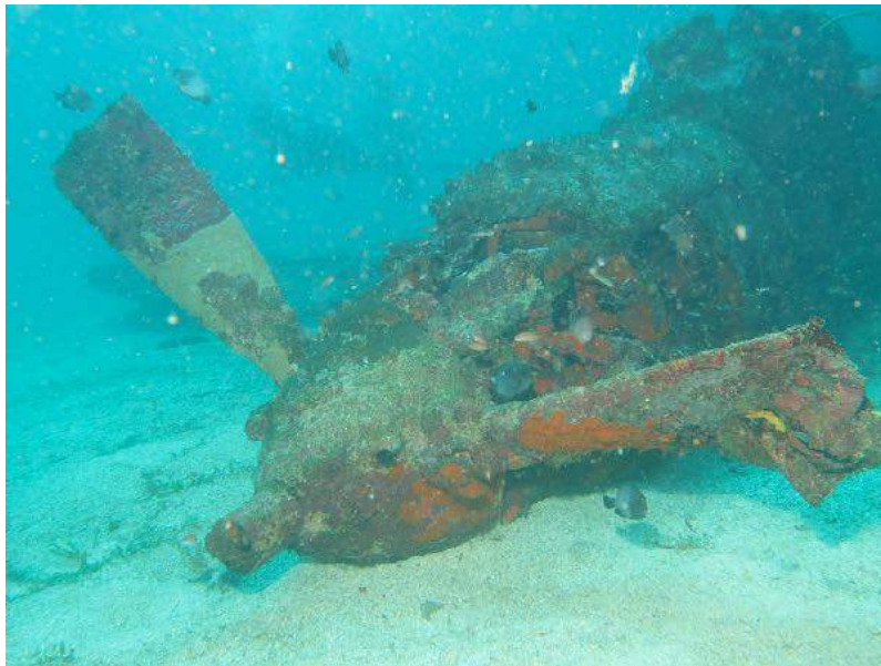
The front of the P-39 shows the prop and 37 mm cannon with its barrel extending through the center of the prop and engine almost back to the cockpit.
