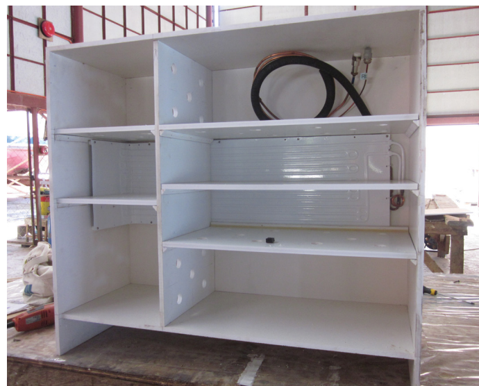
Above, McCampbell's eight-cubic-foot front opening refrigeration box under construction with evaporator plate and shelving in place. Left, this cold box shows an evaporator plate with stand offs. Note tightly-fitted blue solid insulation.
