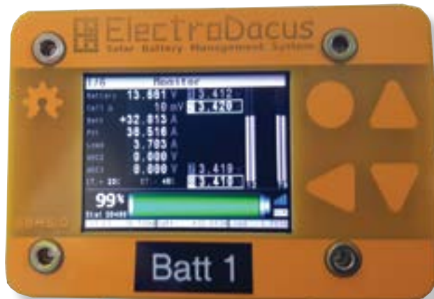
Electrodacus SBMS0 BMS home screen; one of about 20 available screens with all settings adjustable.
