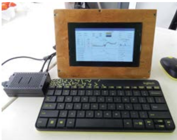
Left, a small Raspberry Pi device running Mosquitto Broker, a Node Red system, and a custom display. Below, the Node Red full display screen.
