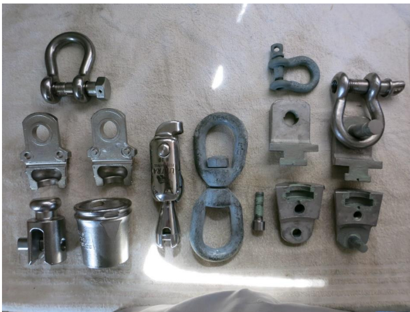
Anchor swivel types (left to right): disassembled Mantus, Ultra ball and socket Flip, Chinese galvanized 5/8" bail to bail, disassembled Kong. All have suitable ratings for 3/8" G4 chain.
