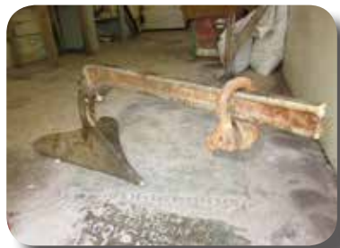
Broken shank on old stainless CQR
