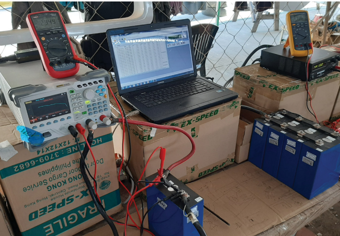
Above, McCampbell put together a testing setup for his recently purchased batteries before installing them in his boat. Right, balancing the cells in parallel.
